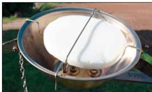
Abb. 16: Sammelmedium Sorbent Impregnated Polyurethane Foam Disk (SIP)
